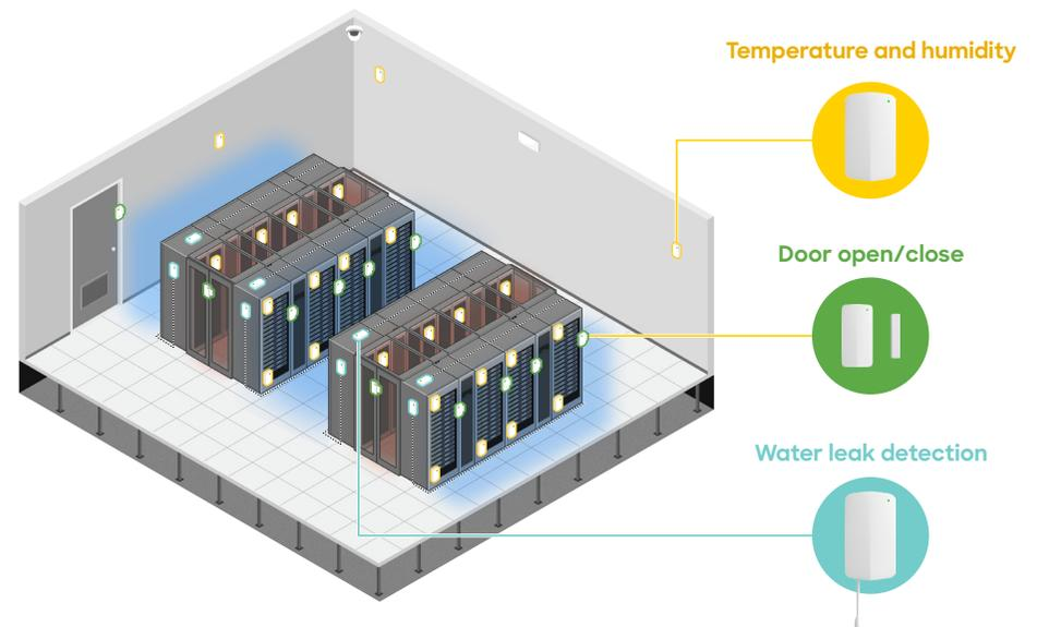
Meraki MT sensors are easy to install and integrate. By placing the sensors strategically, IT teams can reduce the complexity associated with monitoring temperature and humidity while ensuring they stay within the recommended ASHRAE temperature guidelines. Alerts can be sent to key stakeholders when sensor data deviates from the guidelines so issues are quickly remediated.
